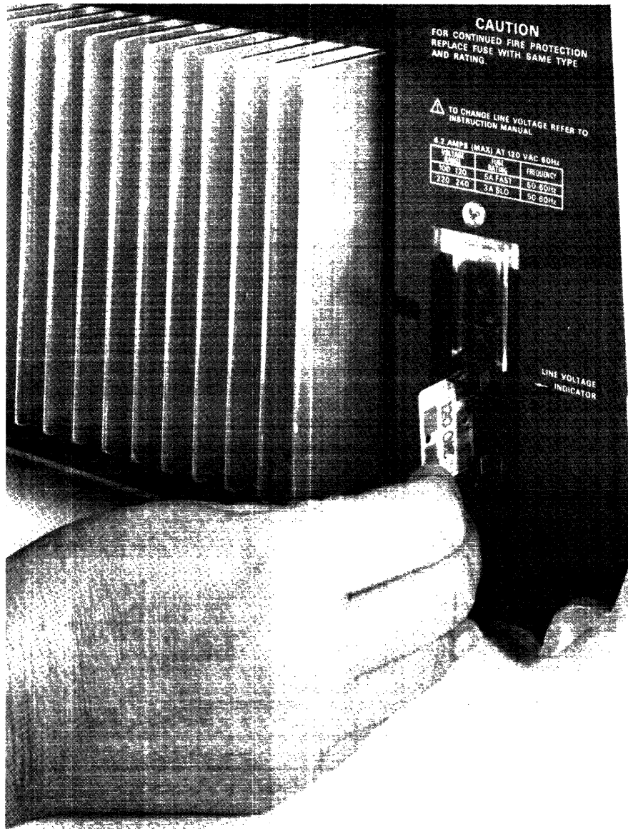
Figure C-15. Inserting the Circuit Card for 120 Vac Selection.
